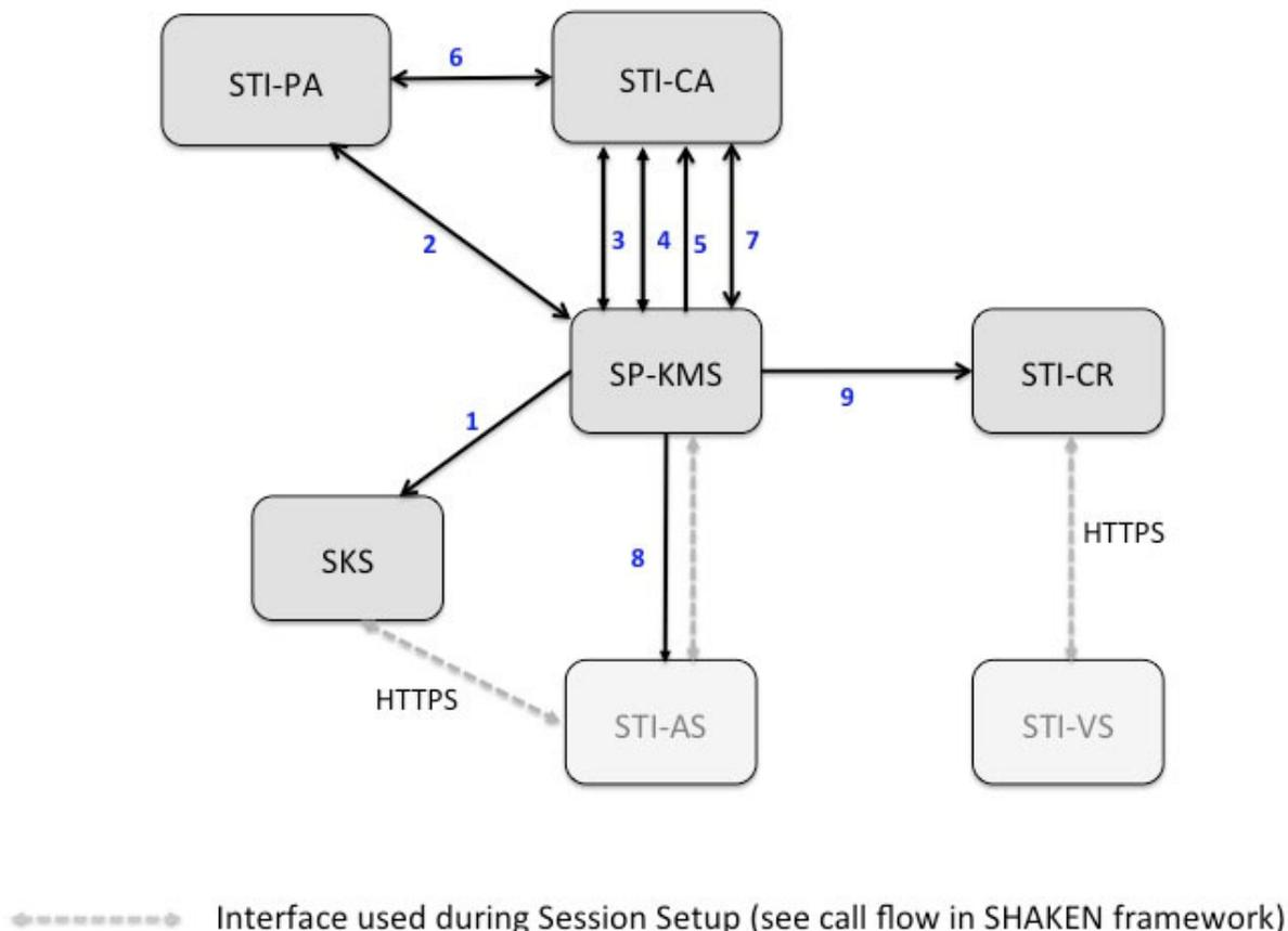
**Figure 6.2 – SHAKEN Certificate Management High Level Call Flow**
