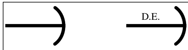
Figure 10: Facility Owner Marking - Terminations/Dead Ends
