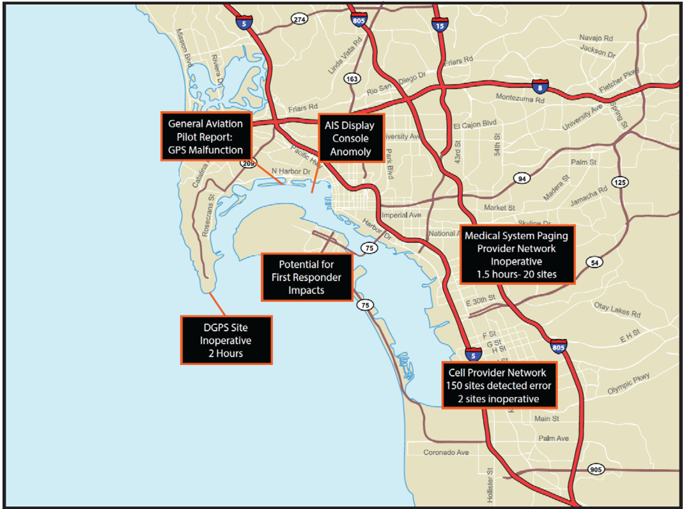
Figure 5.1 – Critical infrastructure disruptions from 2009 U.S. Navy accidental jamming event
